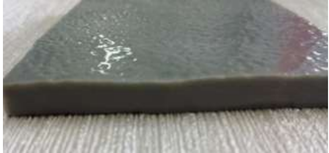
Sample of MTS used to manufacture the new hopper
