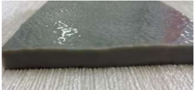
Sample of MTS used to manufacture the new roof.
