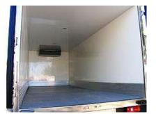
It also provides an aseptic and hygienic environment to vehicles prepared as medical units, providing surfaces: non-slip, smooth, waterproof, washable and resistant to disinfection; or vehicles for the transport of food according to the international agreement ATP-1970.
